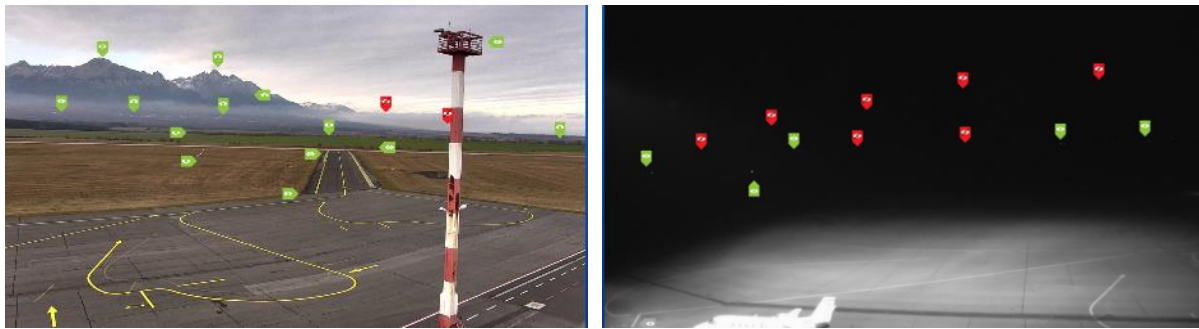
Figure 45: Horizon picture with visibility points for MET Observer during day (left) and night time (right)
